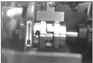
Misalignment is easily detected with a straight edge and using a .005 feeler gage on top and side of coupling will give ample alignment.
